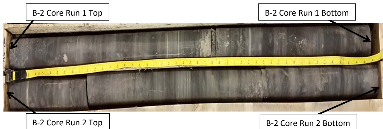
Photograph 8: Top Row: Boring B-2 Core Run 1 (62.0' – 67.0') Second Row: Boring B-2 Core Run 2 (67.0' – 72.0') See Photograph Nos. 9 through 14 for detailed views.
