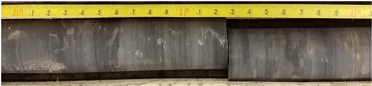
Photograph 6: B-1 – Middle of Core Run 2 – 33.2' – 35.2'.
