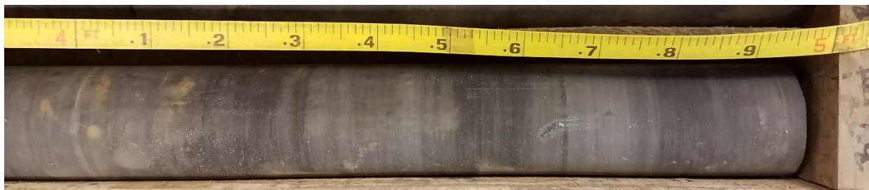
Photograph 4: B-1 – Bottom of Core Run 1 – 30.2' – 31.2'.
